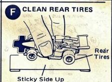
One very effective way to clean tires is to place a piece of tape on a table as shown and roll rear tires on it a few times.
